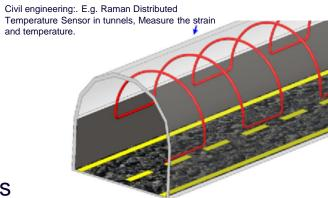
Sensing strain, temperature, pressure, smoke, gas
